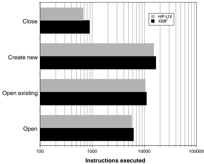
Figure 12: Instructions executed while opening and closing files.
